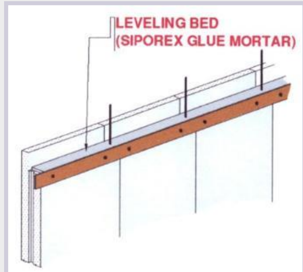
h) Siporex glue is used as leveling bed at top. Dowel bars are positioned for next level.
