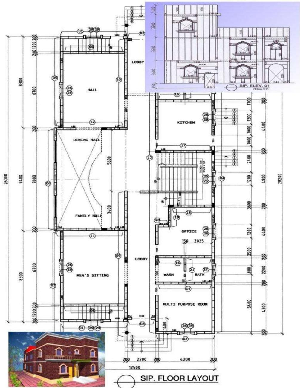
Sample Siporex shop drawings developed from client's architectural plans
